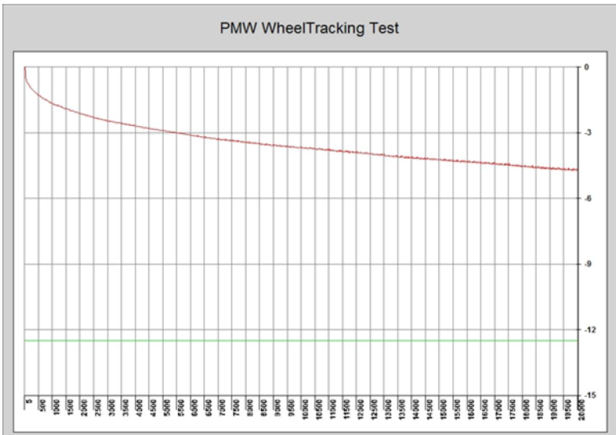
Figure 1: Irwin Control Rut Depth Chart per wheel pass
