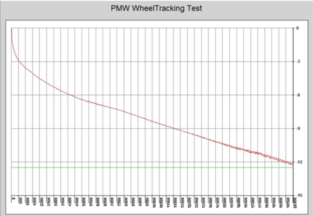
Figure 2: Irwin Bridge Overlay rut depth chart per wheel pass
